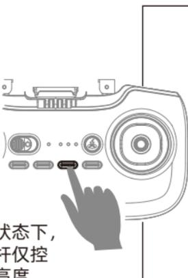
A line drawing of a hand pressing the Orbit mode button on the remote control. The button is located on the right side of the remote, between the mode selector and the power button. The remote control has a large circular dial on the left and several buttons on the right.
